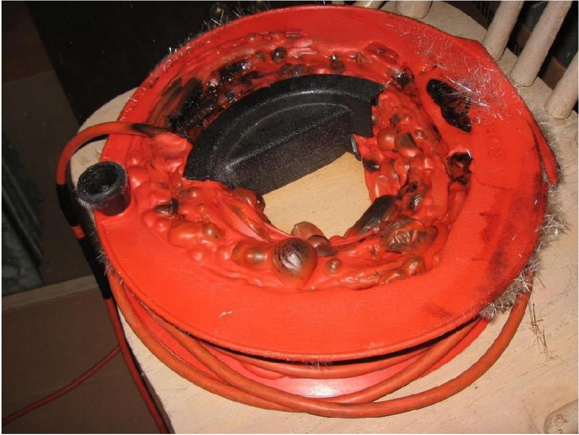
FIGURE 4 COILED WIRES UNDER LOAD MAY OVERHEAT.
