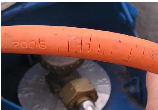
FIGURE 7 PERISHED PIPES OR OLD PIPES WILL FAIL INSPECTION
