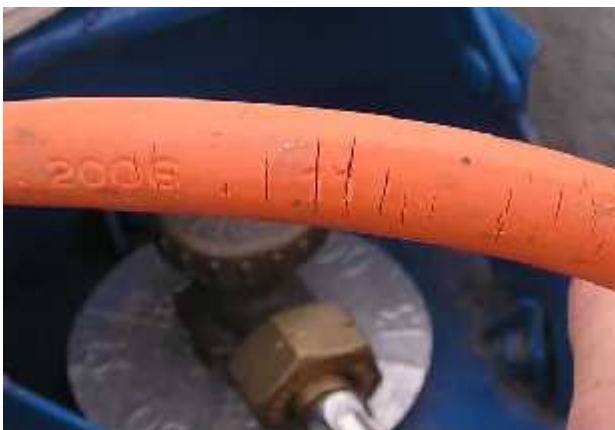
FIGURE 8 PERSIHED PIPES OR OLD PIPES WILL FAIL INSPECTION
