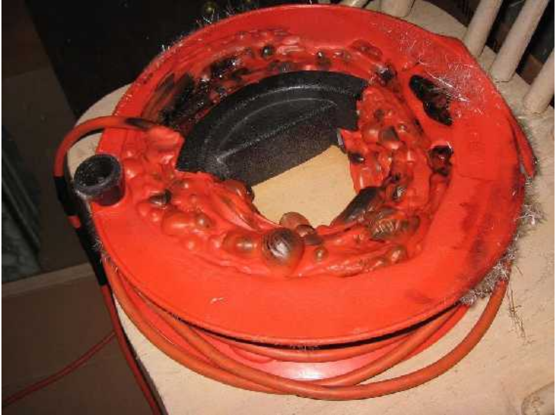
FIGURE 5: COILED WIRE WILL HEAT UP UNDER LOAD AND MAY CATCH FIRE
