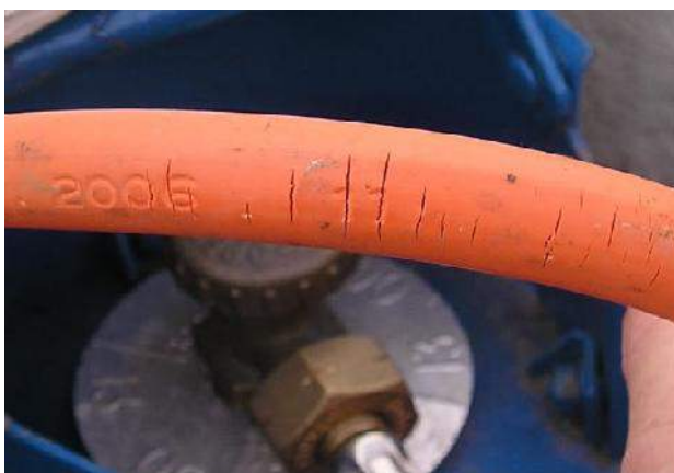
FIGURE 10 PERISHED PIPES OR OLD PIPES WILL FAIL INSPECTION
