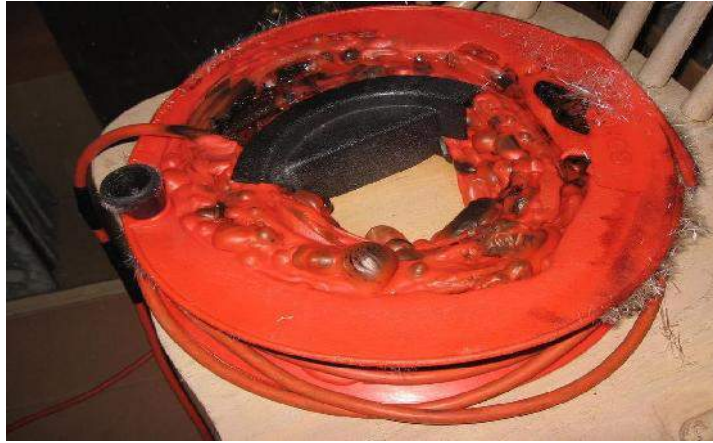
FIGURE 6: COILED WIRE WILL HEAT UP UNDER LOAD AND MAY CATCH FIRE
